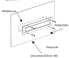
Use proper 8/32 or M5 screws according to the application and material where the fixture is set up. Choose screws length with relation to the thickness of the material (Pic. 4). ENGLISH Plug-in
